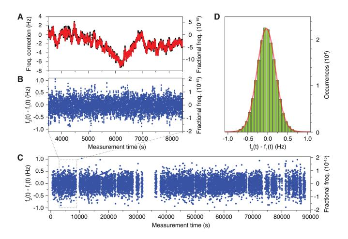
**Fig. 2.** (**A**) Correction frequencies,  $f_{1,2}(t)$ , are shown in red and black. Dominant LO fluctuations are due to the cavity and are thus common to the atomic systems. (**B**) Frequency difference between the two Yb clock systems,  $f_2(t) - f_1(t)$ , for a 5000 s interval. (**C**) Data set  $f_2(t) - f_1(t)$  over a 90,000 s interval. Gaps represent data rejected before data analysis due to servo unlocks. (**D**) A histogram of all data and a Gaussian fit  $(\chi^2_r = 0.9996)$ .
