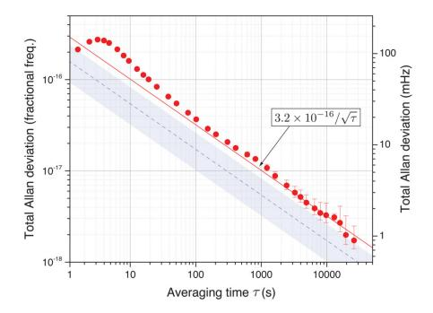
**Fig. 3.** Total Allan deviation of a single Yb clock,  $\left(f_2(t)-f_1(t)\right)/\sqrt{2}$  (red circles), and its white-frequency-noise asymptote of  $3.2\times10^{-16}/\sqrt{\tau}$  (red solid line). The blue dashed line represents the estimated combined instability contributions from the Dick effect  $\left(1.4\times10^{-16}/\sqrt{\tau}\right)$  and QPN  $\left(1\times10^{-16}/\sqrt{\tau}\right)$ ; the shaded region denotes uncertainty in these estimates.
